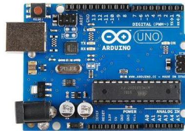
**Fig.2 Arduino Uno Board [9]**
