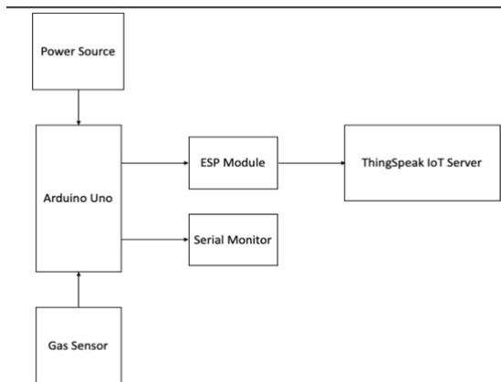
Fig.5 Hardware circuit flowchart
