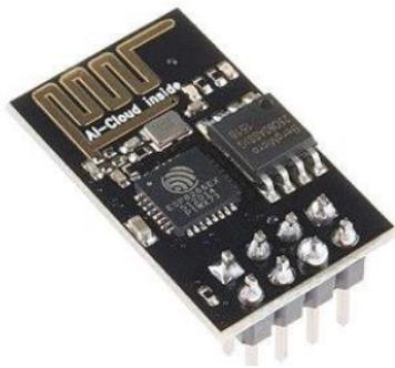
Fig.3 ESP8266 Board [10]
